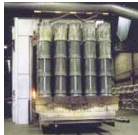
Wagonnets de four
